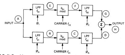
Fig. 3 Schematic of Split Band Inverter
