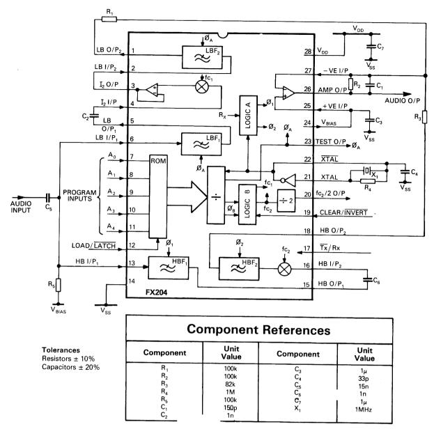
Fig. 2. External Component Connections
