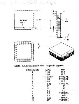
FX204J28-pin cerdip DILFX204LH28-lead plastic leaded<br/>chip carrier.
